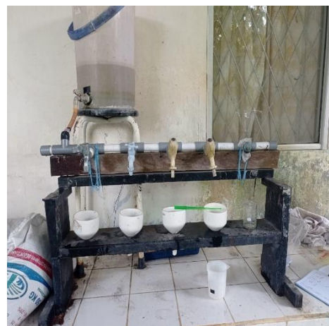
Figures 5 and 6. Analysis of soil permeability in the laboratory
