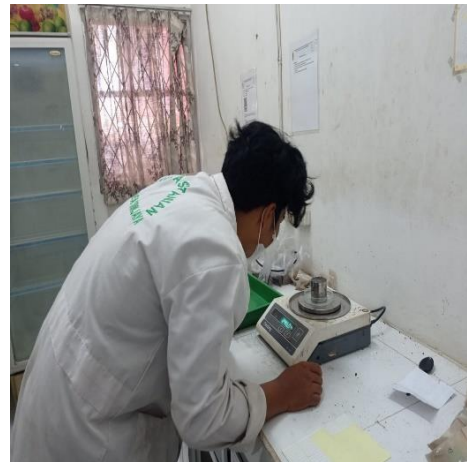
Figures 3 and 4. Analysis of bulk density and total soil pore space
