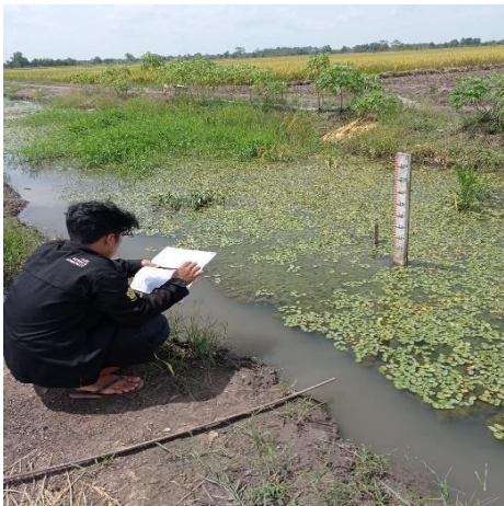
Figures 3 and 4. Observation of water level in canals and groundwater level
