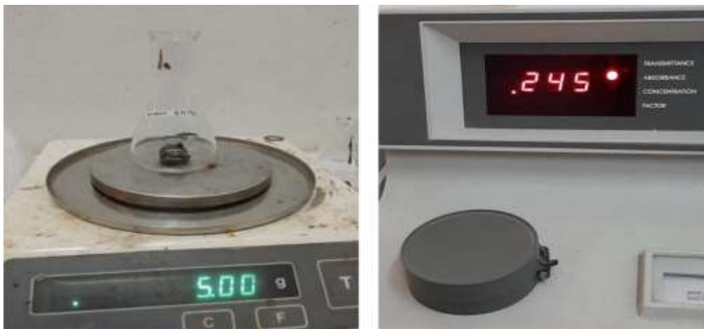
Photo 8. Observing the Value of Dissolved Fe, Dissolved Sulfate Using Spectrophotometer
