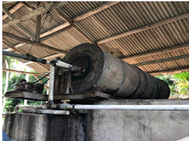
Figure 4.9. Dregs Separator Machine
