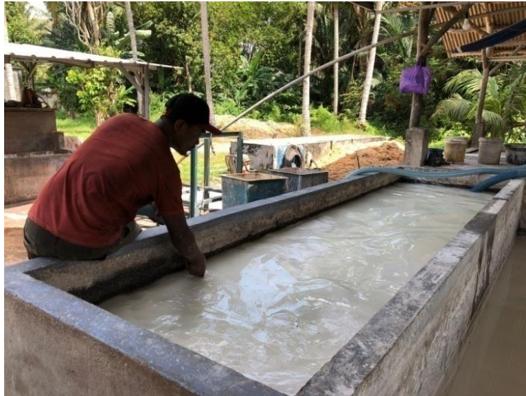
Figure 4.33. Second Precipitation in Sago Palm
