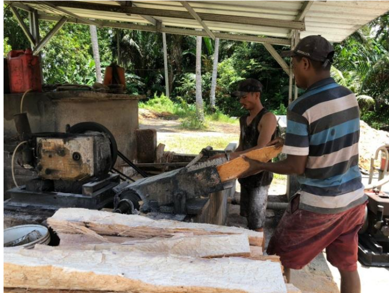
Figure 4.30. Grate Tatch Stem with Grate Machine
