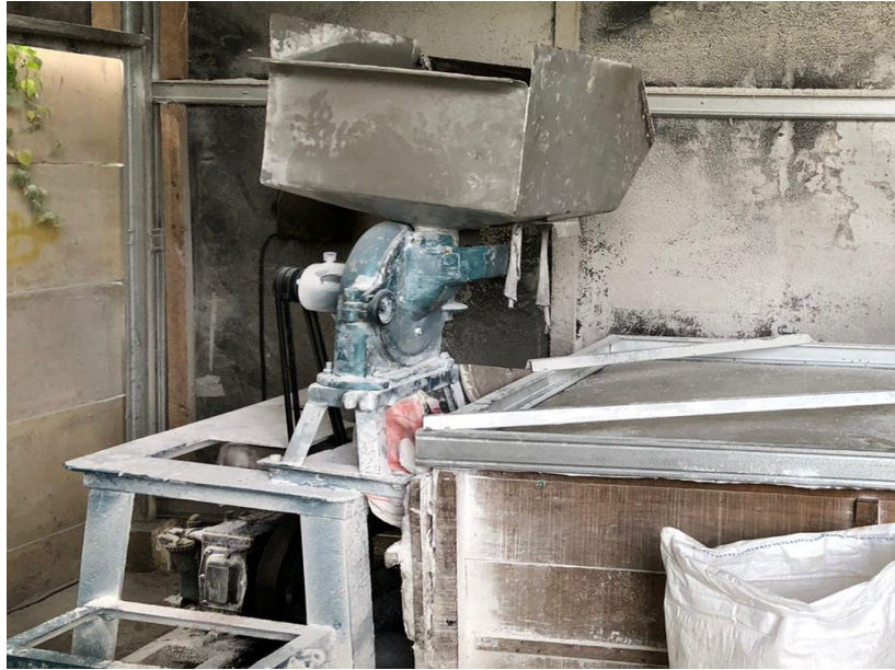
Figure 4.13. Dry Sago Milling Machine
