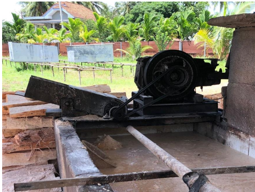
Figure 4.11. Thatch Stem Grate Machine
