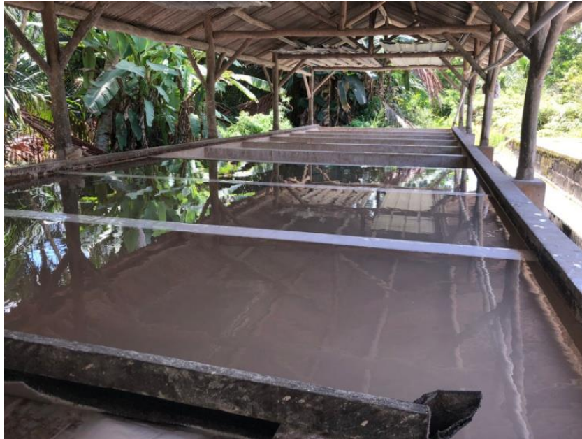
Figure 4.32. First Precipitation on Sago Palm
